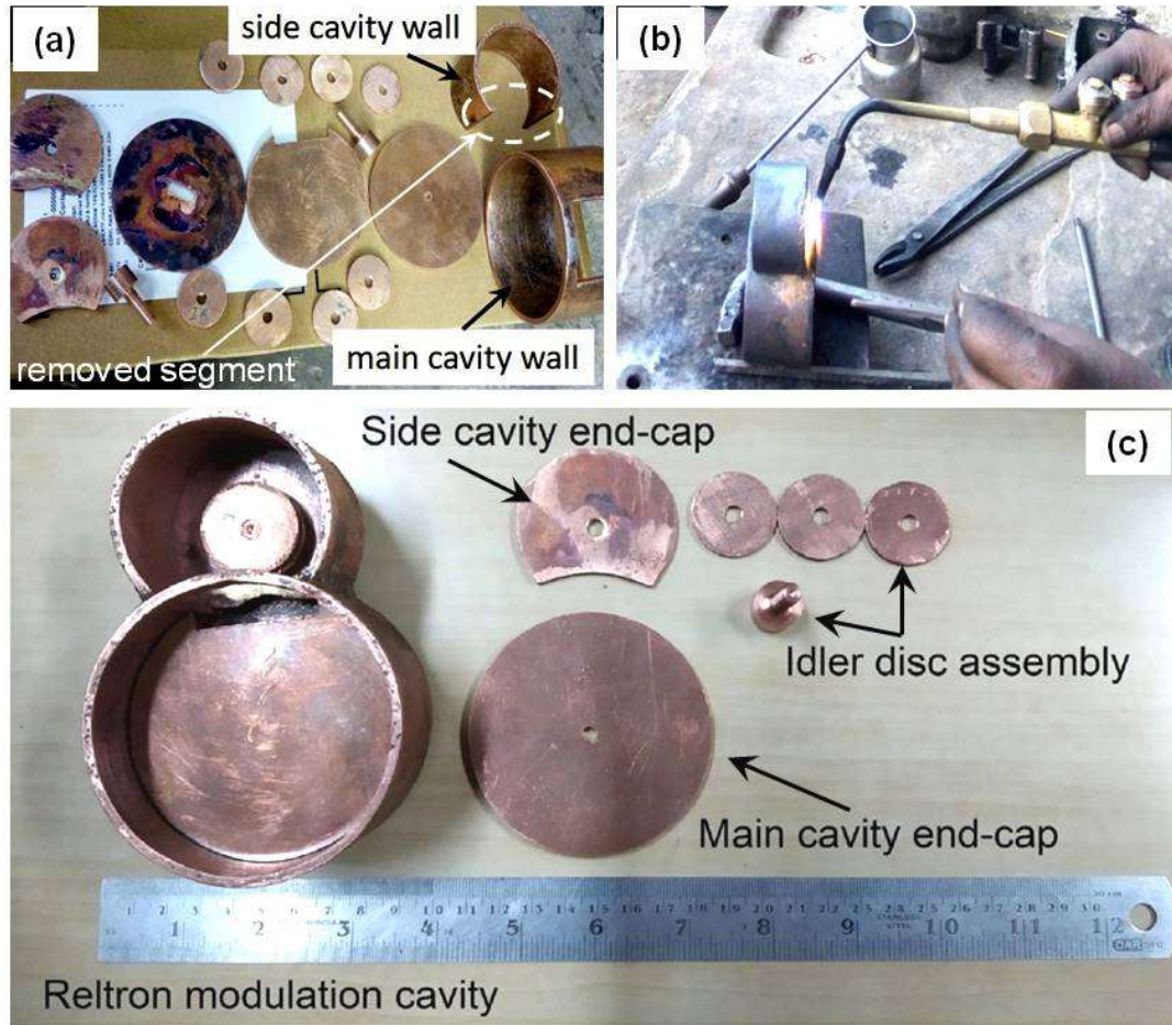
Figure 2.10: Construction of reltron modulation section showing– (a) different parts of the cavity, (b) the main cavity being joined with the side cavity by gas welding, and (c) final structure.
