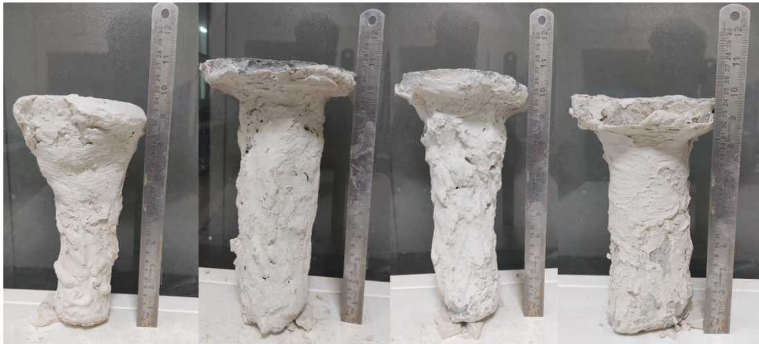
Fig. 5.16 Typical lateral deformation/bulging of (25% TC + 75% AG) (a) OGP, (b) VEGP,(c) HEGP-0.25D,and (d) CEGP-0.25D.
