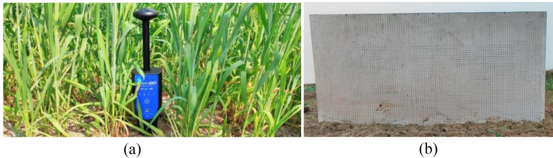
Figure 2.1 Illustration of measurement of (a) soil moisture through HydraGO device and (b) surface roughness employing plate insertion technique
