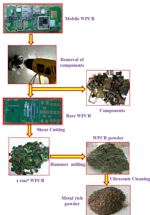
Figure 2.1-Schematic representation of proposed experimental procedure of WPCBs pre-treatment
