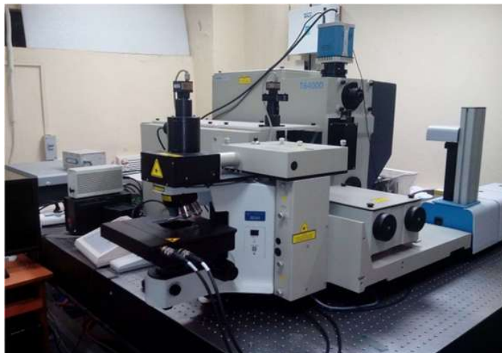
Figure 2.11 Experimental set-up used for Raman Measurement (CRF IIT Kharagpur).
