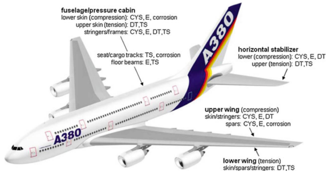
FIGURE 1.2: Engineering properties required for main structural components [4].
