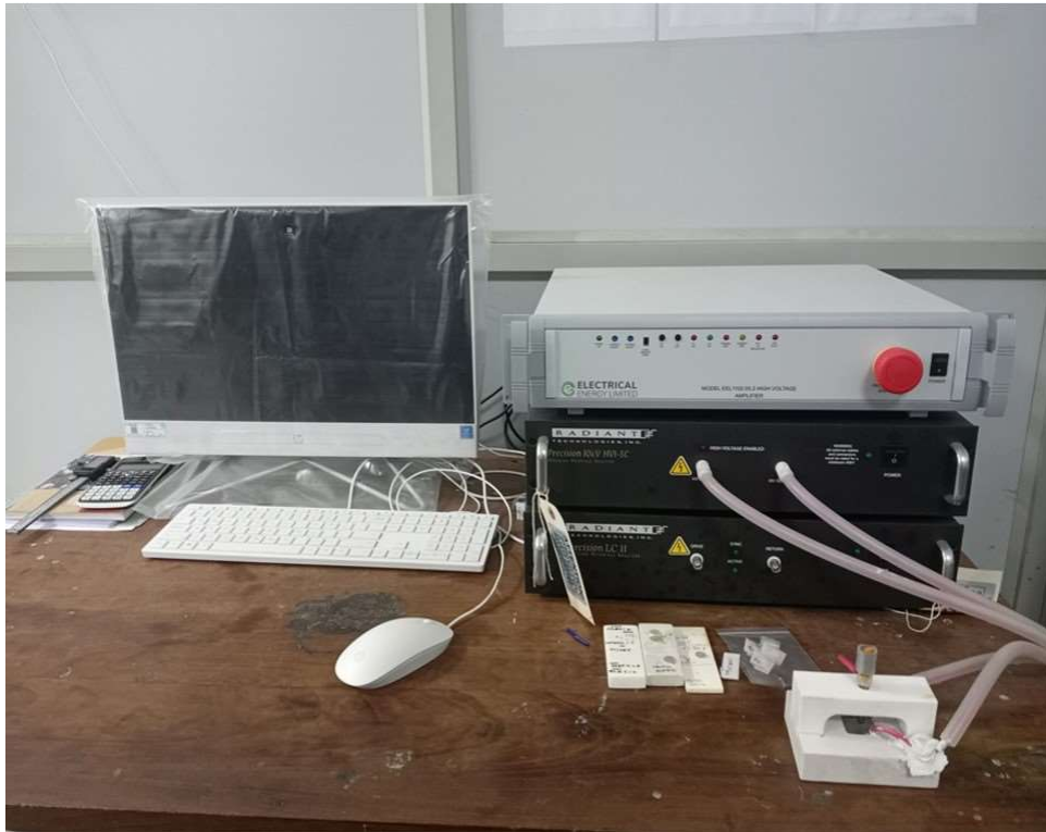
Fig. 2.7 Polarization vs. electric field (PE) hysteresis loop tracer (Radiant Inc.).
