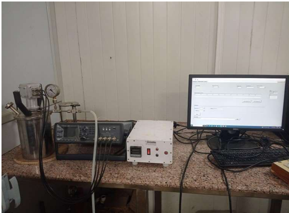
Fig. 2.6 LCR meter along with variable temperature stage for dielectric measurements.
