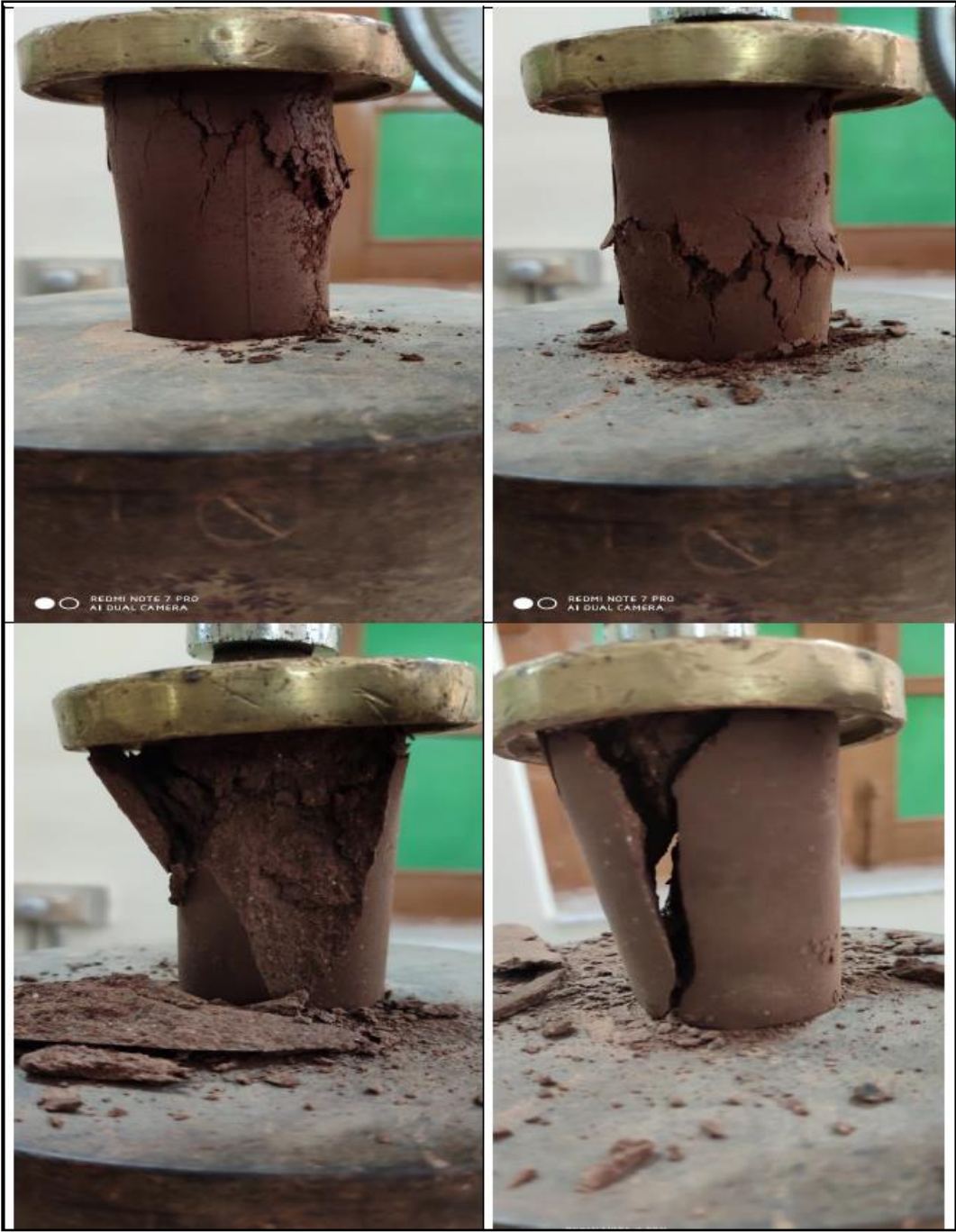
Fig: 6.6 UCS Testing of Red mud-GGBFS Mixes
