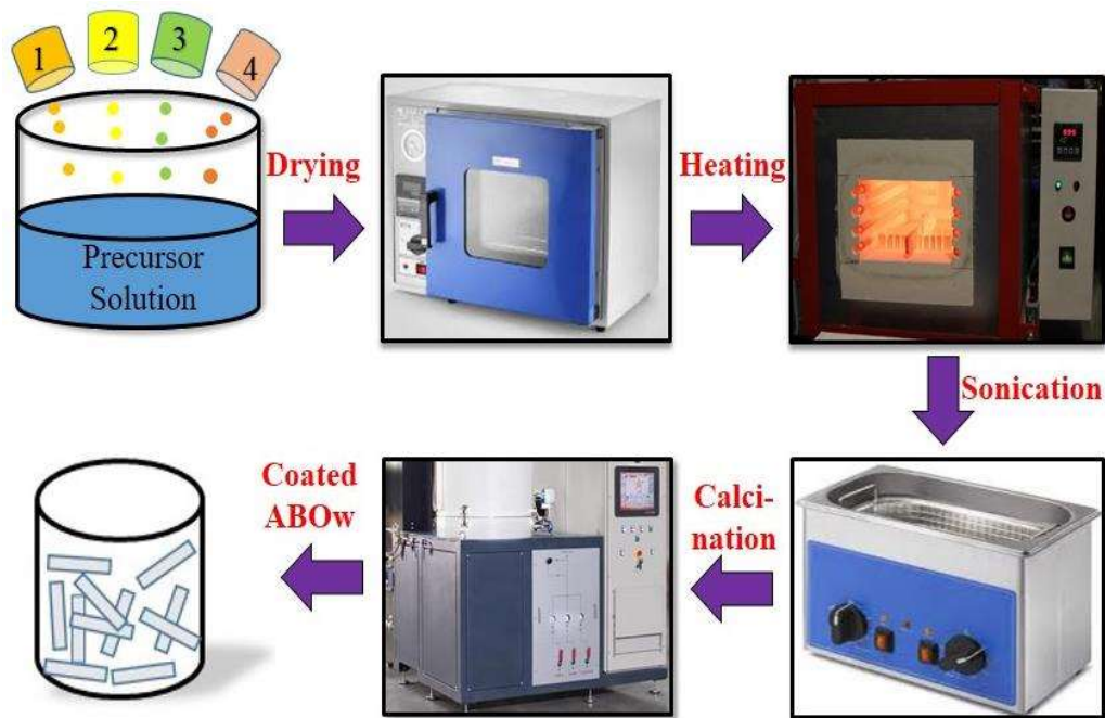
Figure 3.2: (a) Mixing (b) Oven (c) Furnace (d) Sonication (e) Heating (f) Coated ABO w
