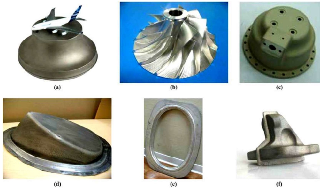
Figure 2. 5: (a) AZ80 compressor wheel produced by closed-die forging; (b) WE43 impeller with twisted blades; (c) WE43 compressor upper case for air conditioning system produced by closed- die forging; (d) AZ31B euro copter antenna support produced by deep drawing; (e) AZ80- forged airbus window frame; (f) AZ80- forged door stop fitting [38]
