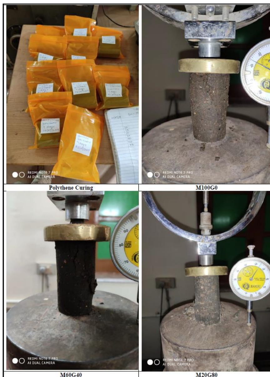
Fig: 5.6 Sample preparation and UCS Testing
