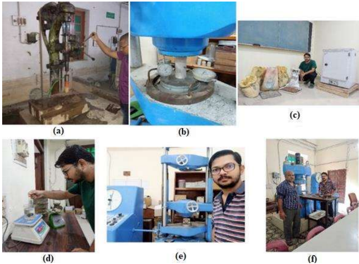
Fig. 4.15. Laboratory tests on rock samples (a) Sample preparation (b) Poisson's ratio (c) Sample collected from sites (d) Specific gravity (e) Brazilian tensile and (f) Triaxial test
