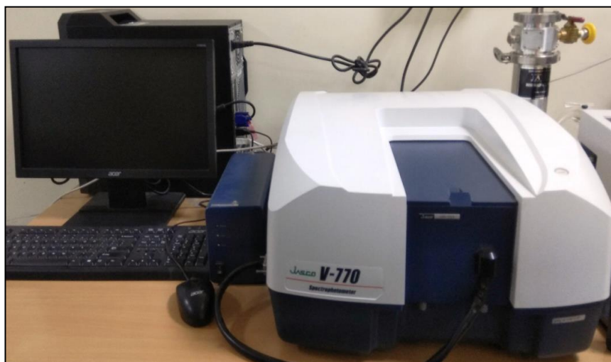
Figure 2.9 Experimental setup of UV-Visible measurement [JASCO V-770 UV-Vis spectrophotometer].
