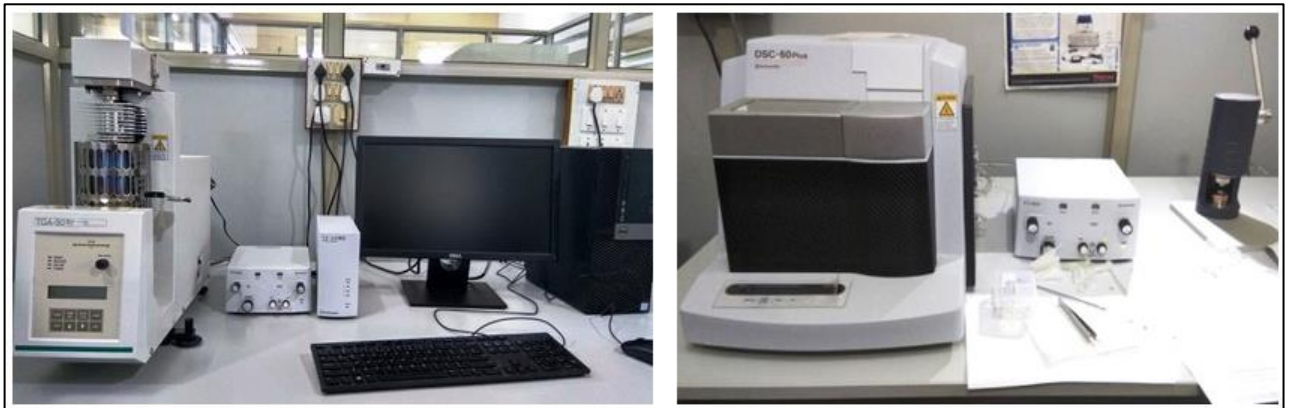
Figure 2.4 The experimental setup of TGA/DSC.
