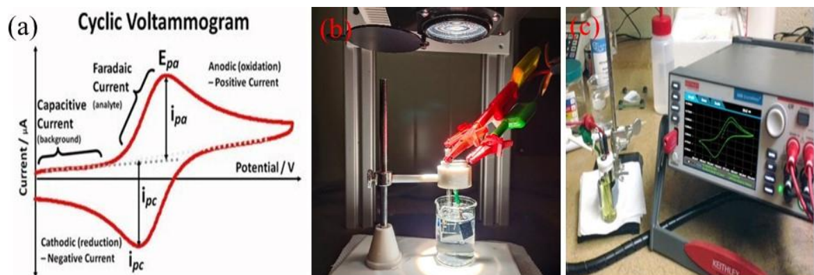
Figure 2.13: Schematic representation of (a) typical CV curve, (b) photoelectrochemical cell setup using CV at our laboratory, and (c) the CV setup.
