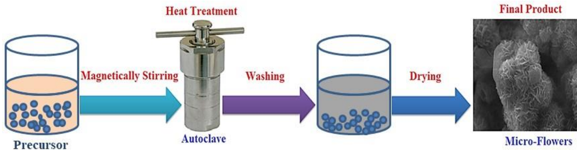
Figure 2.3: Schematic diagram of hydrothermal synthesis method [65].
