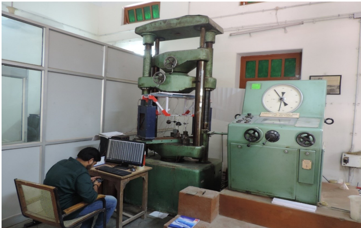
Figure 3.22 Setup for the composite model test, showing UTM, data logger and mounted strain gauges.
