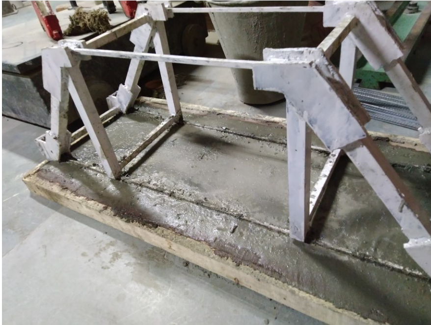
Figure 3.19 Inverted model in the mold for deck slab casting
