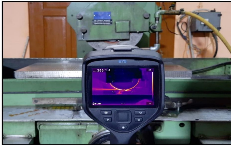
Fig. 3.8: Temperature measurement arrangement during grinding.
