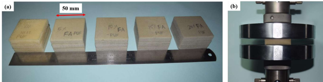
Figure 3.13 (a) PUF core compression test coupons arranged in increasing wt.% of FA reinforcement neat, 5%, 10%, 15% and 20% respectively (b) PUF specimen under compression test configuration.
