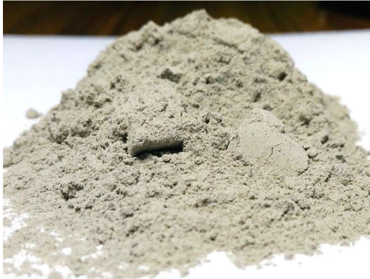
Figure 3.7 Micro-sized fly ash particles used as filler in PU foam core
