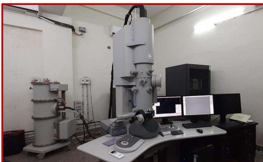
Figure 2.4 Transmission electron microscopy (FEI Technai-20 G 2 ).
