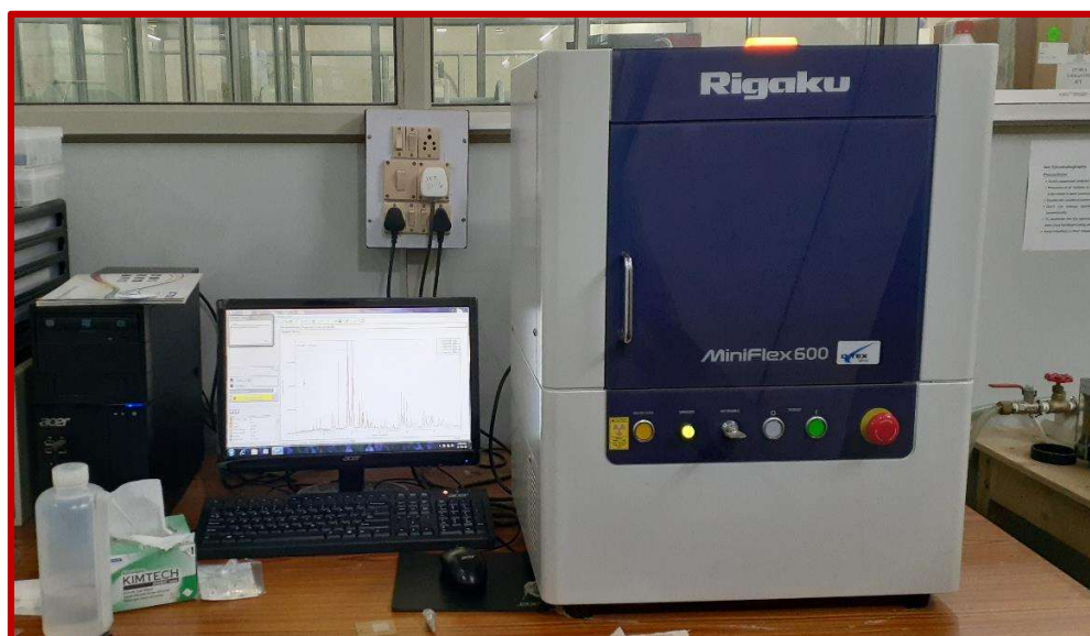
Figure 2.2 XRD diffractometer (Mini Flex 600).
