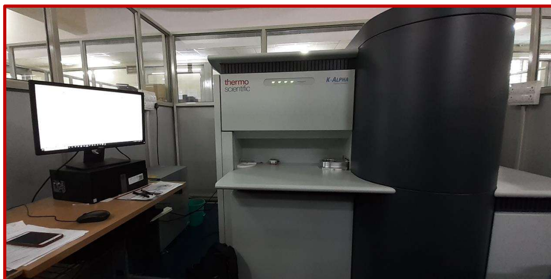
Figure 2.5 X-ray photoelectron spectroscopy (Thermo fisher scientific make K-Alpha).
