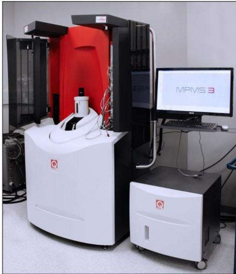
Figure 2.6 MPMS-3, Quantum Design (USA) used for magnetic measurement
