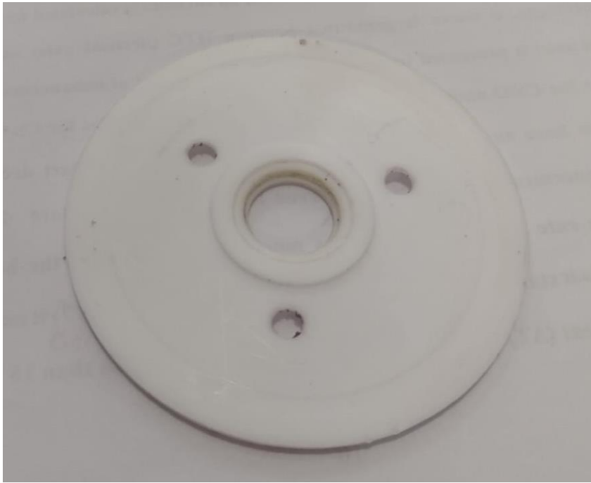
Fig. 4.2. Sample holder made of PTFE Teflon (pictorial view).
