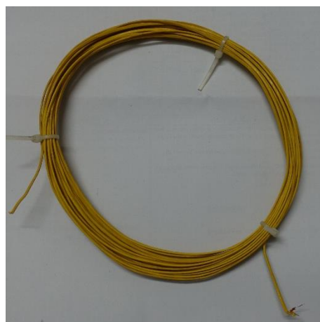
Fig. 4.5. Image of K-type thermocouple (wire diameter 0.3 mm).
