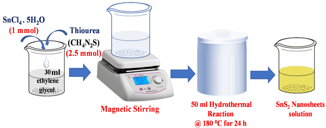
Figure 4.1: Solvothermal synthesis of SnS 2 nanoflakes
