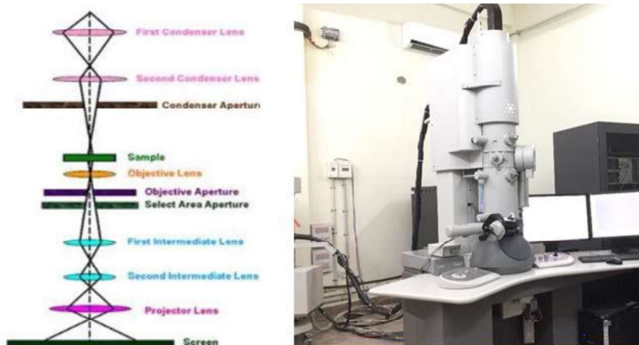
Fig. Appendix(B).0.4 Schematic representation of principle of Transmission electron microscopy (TEM) and Photograph of TEM
