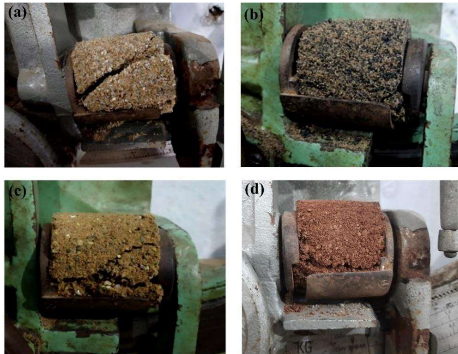
Figure 4.8: Failure of mold during shear test
