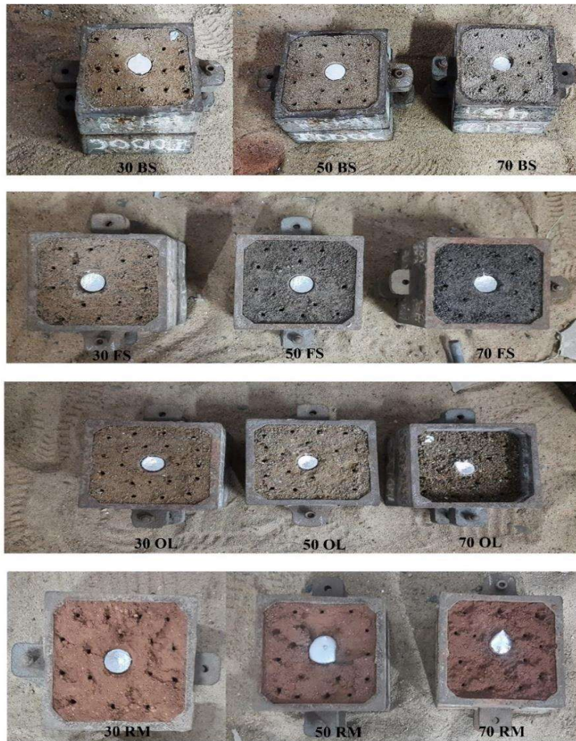
Figure 4.14: Casting of A319 alloy in various mold
