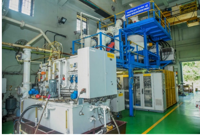
Fig. 4.1: Chemical vapour infiltration (CVI) reactor in VSSC/ISRO.
