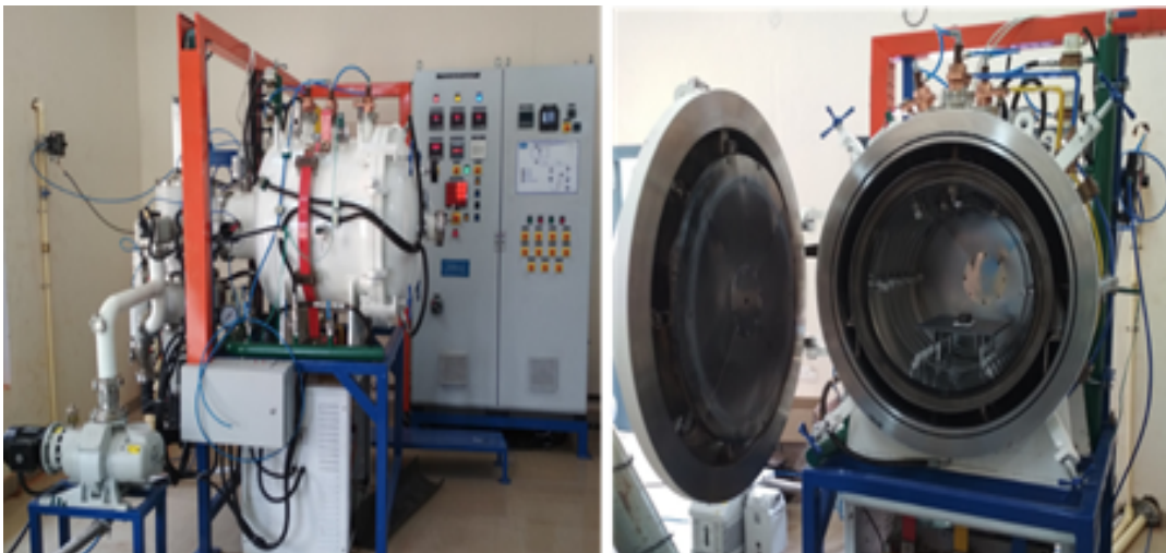
Fig. 4.5: Vacuum brazing furnace.
