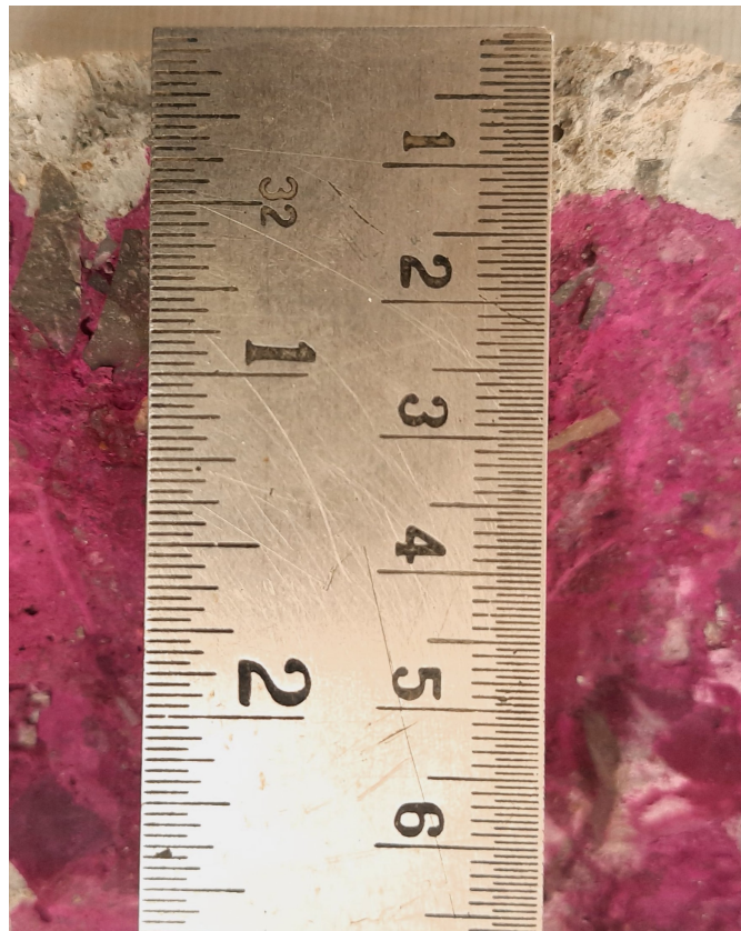
Figure 6.35: Carbonation depth of C60RC
