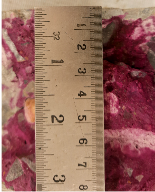
Figure 6.34: Carbonation depth of C30RC
