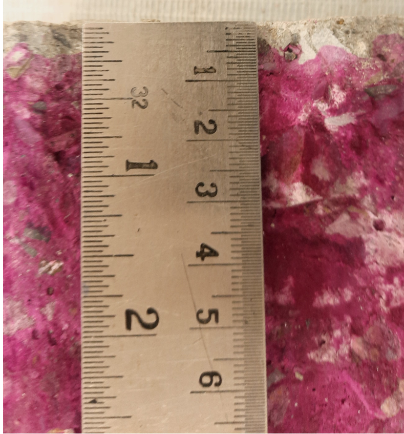
Figure 6.36: Carbonation depth of C100RC
