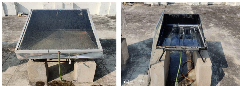
FIGURE 2 Experimental set up of solar still A, without Quantum Dot B, with glass powder Quantum dot
