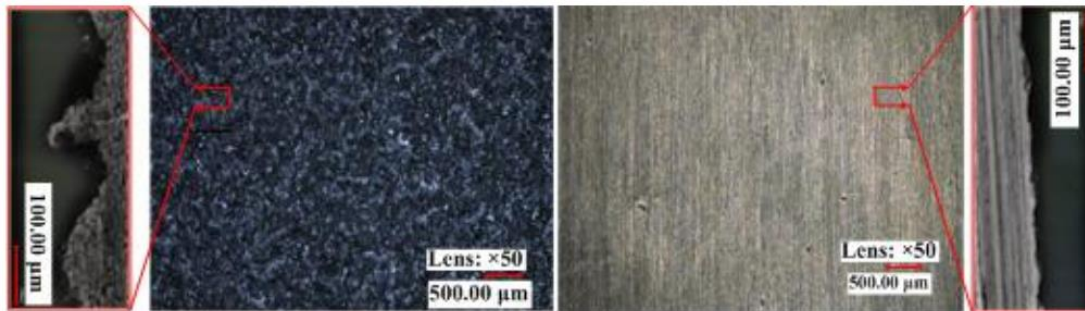
Figure 1.13 Comparison of the as-built and the finished surface after AFM process [94]
