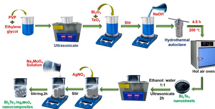
Scheme 1. Schematic presentation for the synthesis of \text{Ag}_2\text{MoO}_4/\text{Bi}_2\text{Te}_3 nanocomposites.
