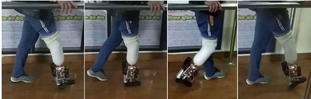
Figure 6.6 Transtibial amputee walking on MR damper-based ankle-foot prosthesis prototype
