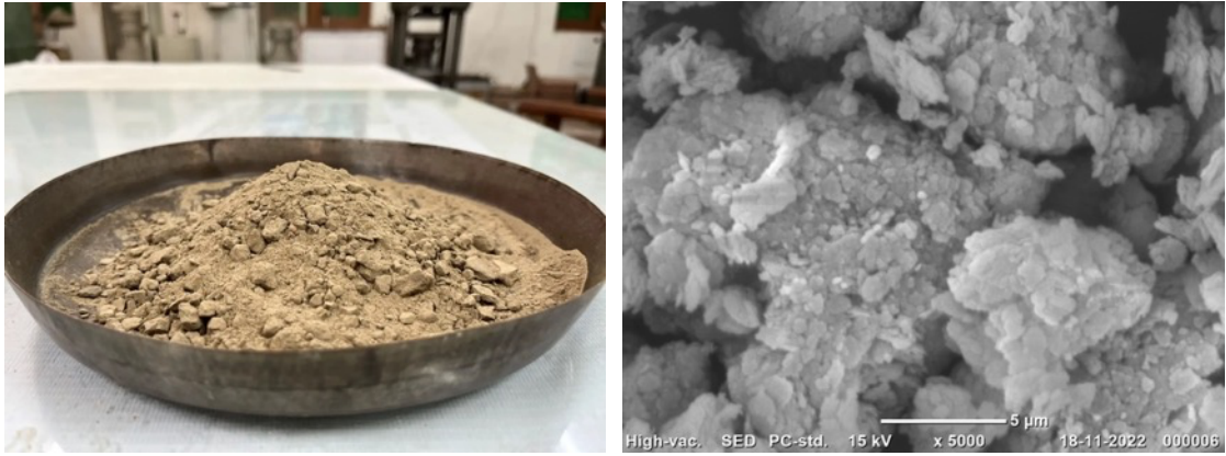
Figure 3.1 (a) Metakaolin and (b) SEM image of metakaolin
