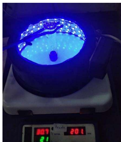
Figure 3.7 A reaction setup showing the reaction tube was fixed at 5-6 cm from the blue LED stripped (80 cm). [Personal photo made by one of the authors- Arsala Kamal]
