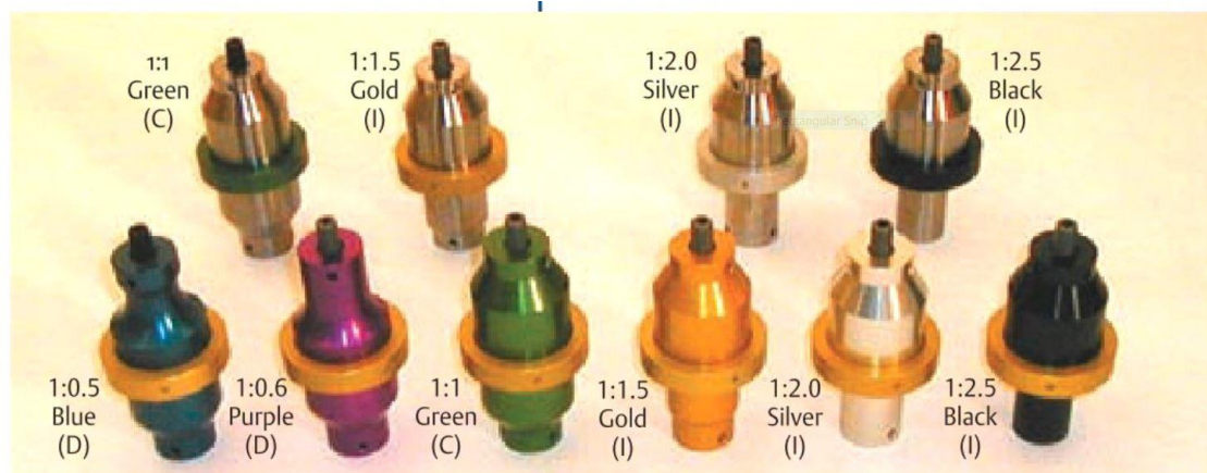
Figure 1.5 Classification of the booster based on seven colour codes and their gain ratio (upper row: titanium and lower row: aluminum) (D = amplitude decreasing; C = coupling, no change; I= amplitude increasing) [79]
