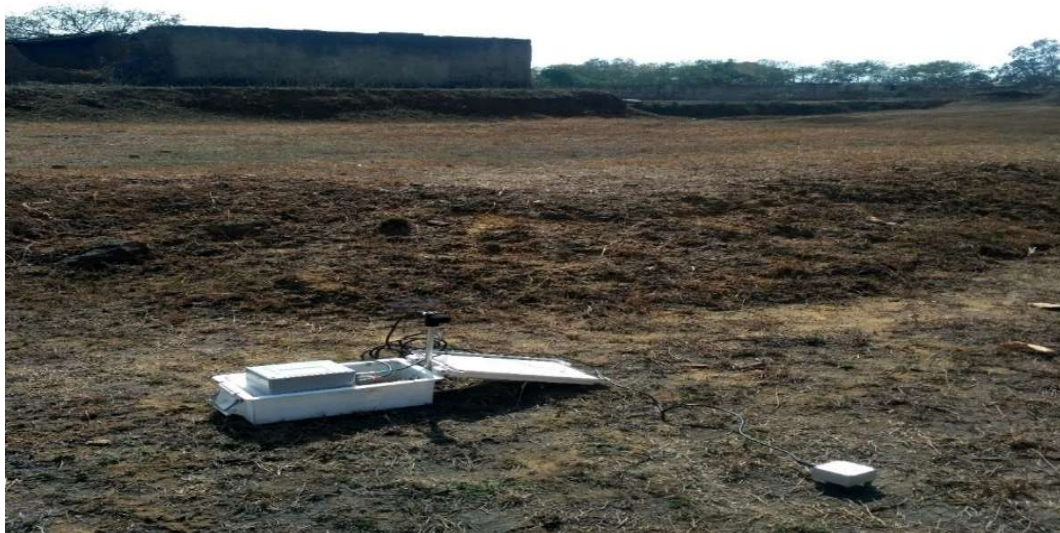
Figure 4.6 Seismograph installed nearby the village.
