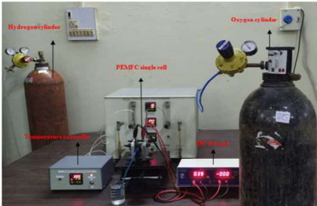
Figure A1 Photographic view of PEMFC single cell experimental setup.
