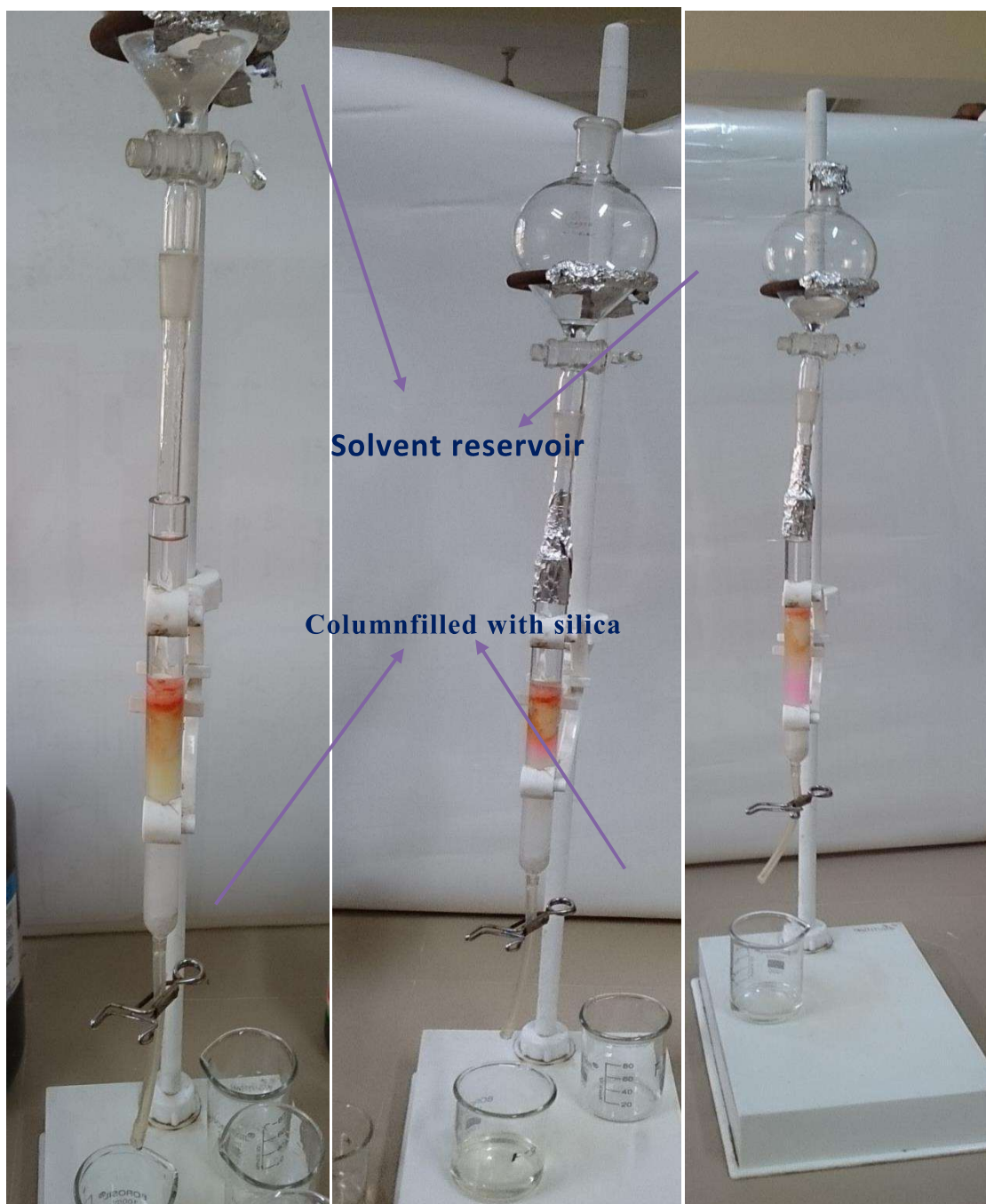
Fig. 6 Different stages of column chromatography during fractionation of crude metabolite
