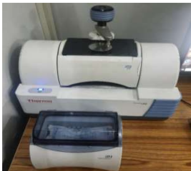
Figure 3.4 Nicolet iS5 spectrophotometer
