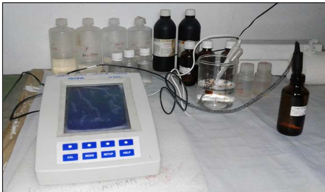
Figure 4.19 Hanna Lab Bench Meter- Hi4222 for analysis of Nitrate & Fluoride
