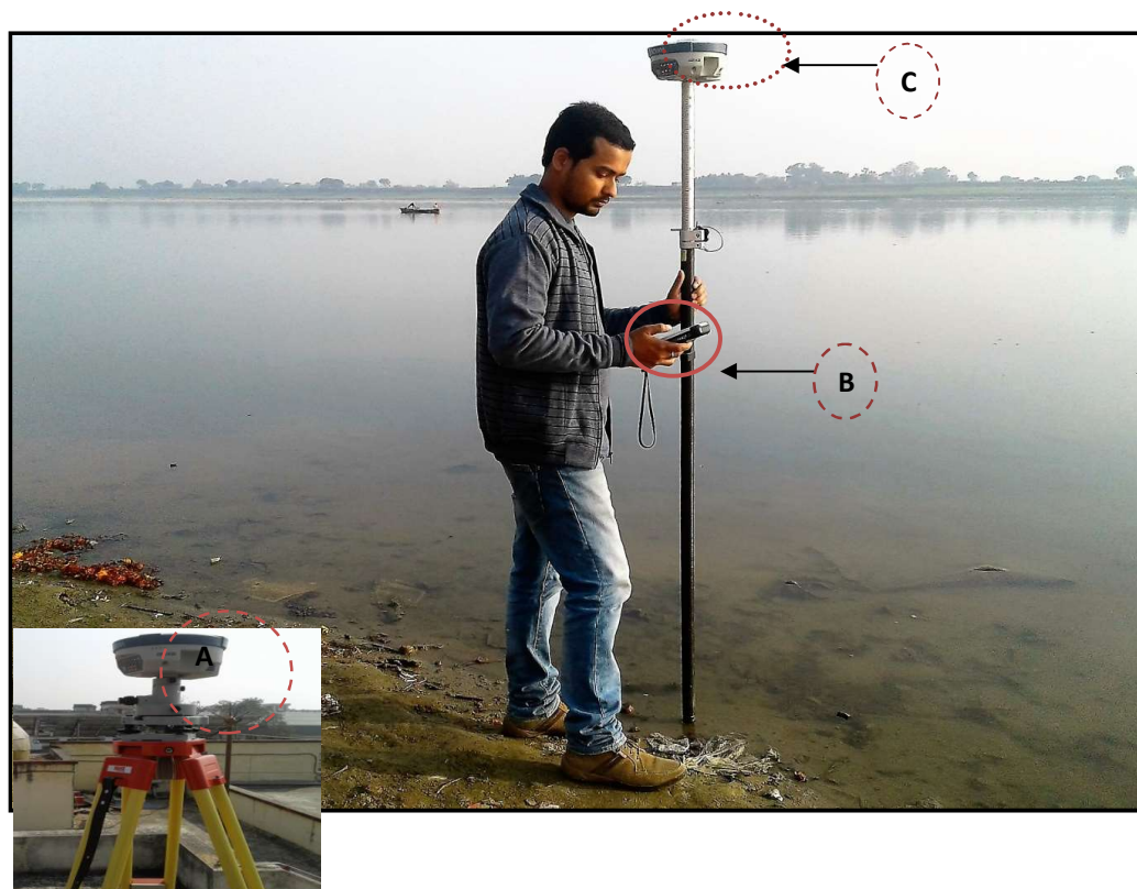
Figure 4.3 DGPS Surveying A) The base station B) Controller (C) Rover
