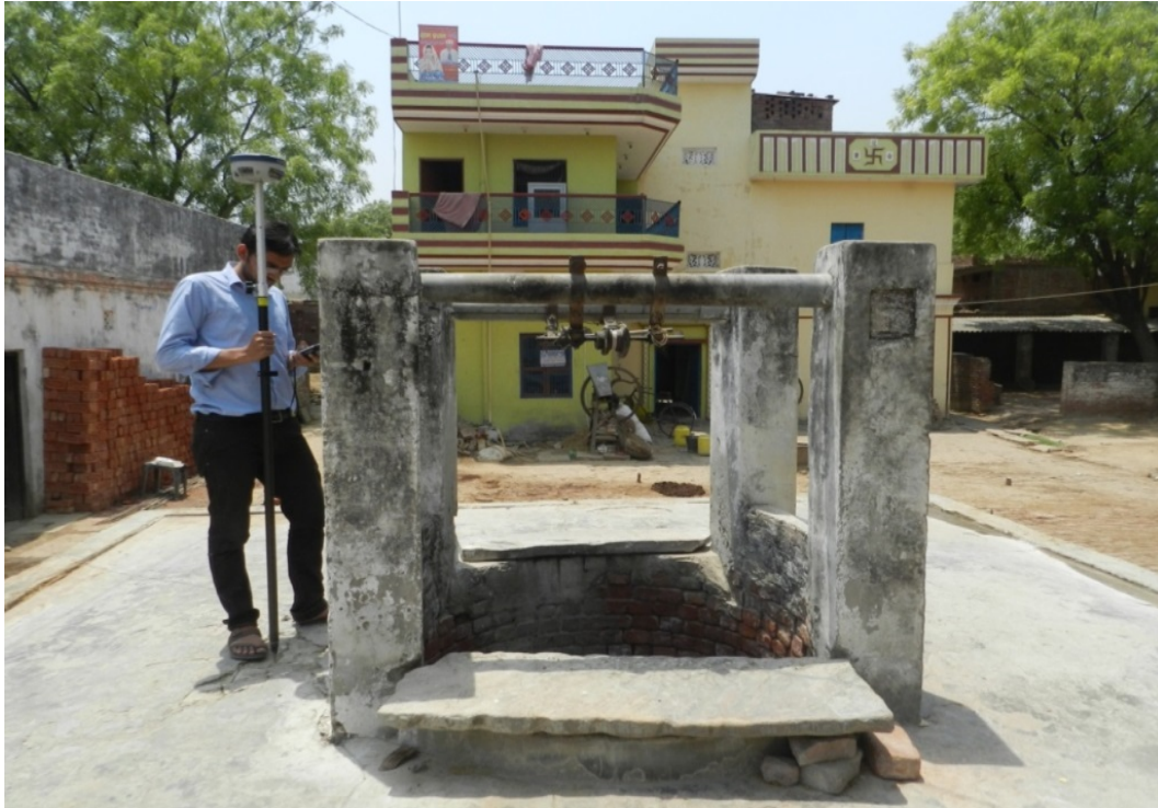
Figure 4.4 Taking geo-location of open well by DGPS
