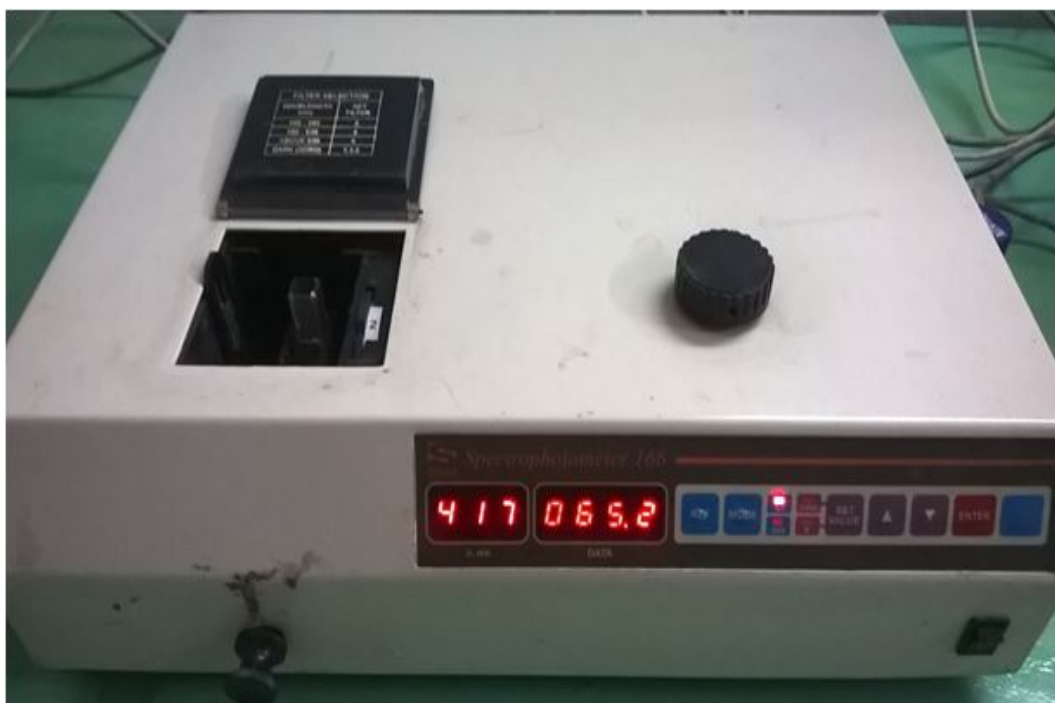
Figure 4.15 Spectrophotometer for phosphate analysis
