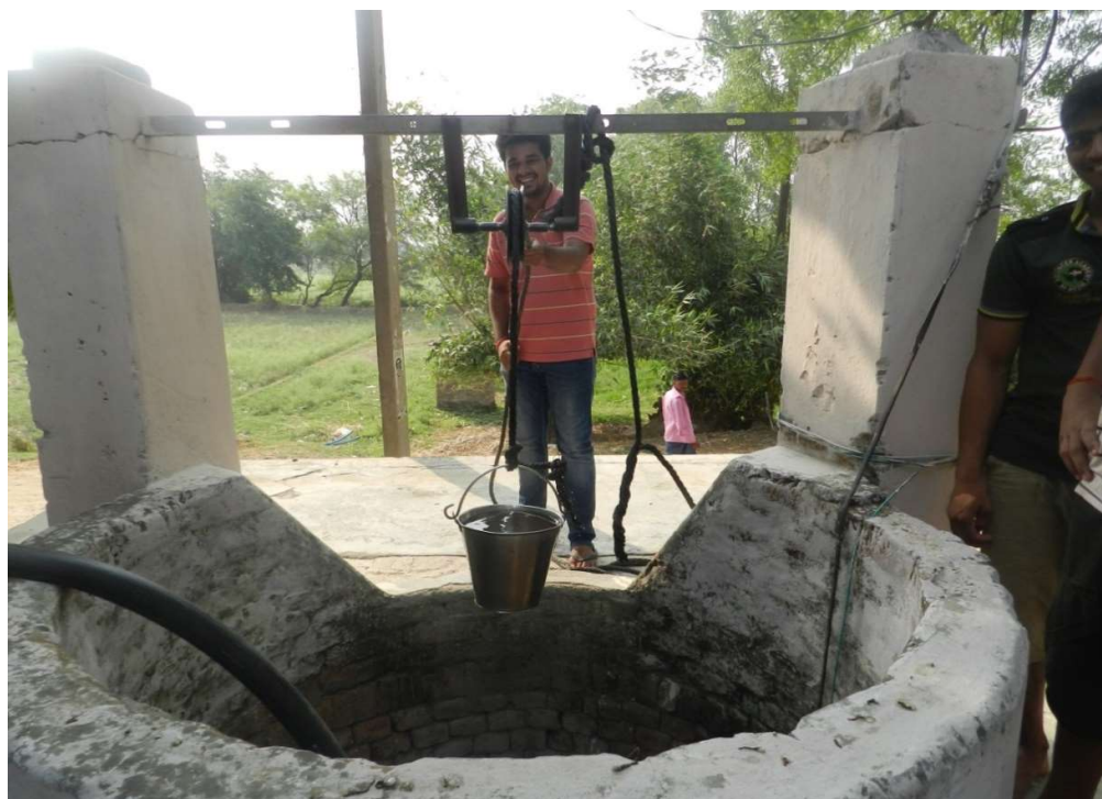
Figure 4.12 open dug well for groundwater sampling
