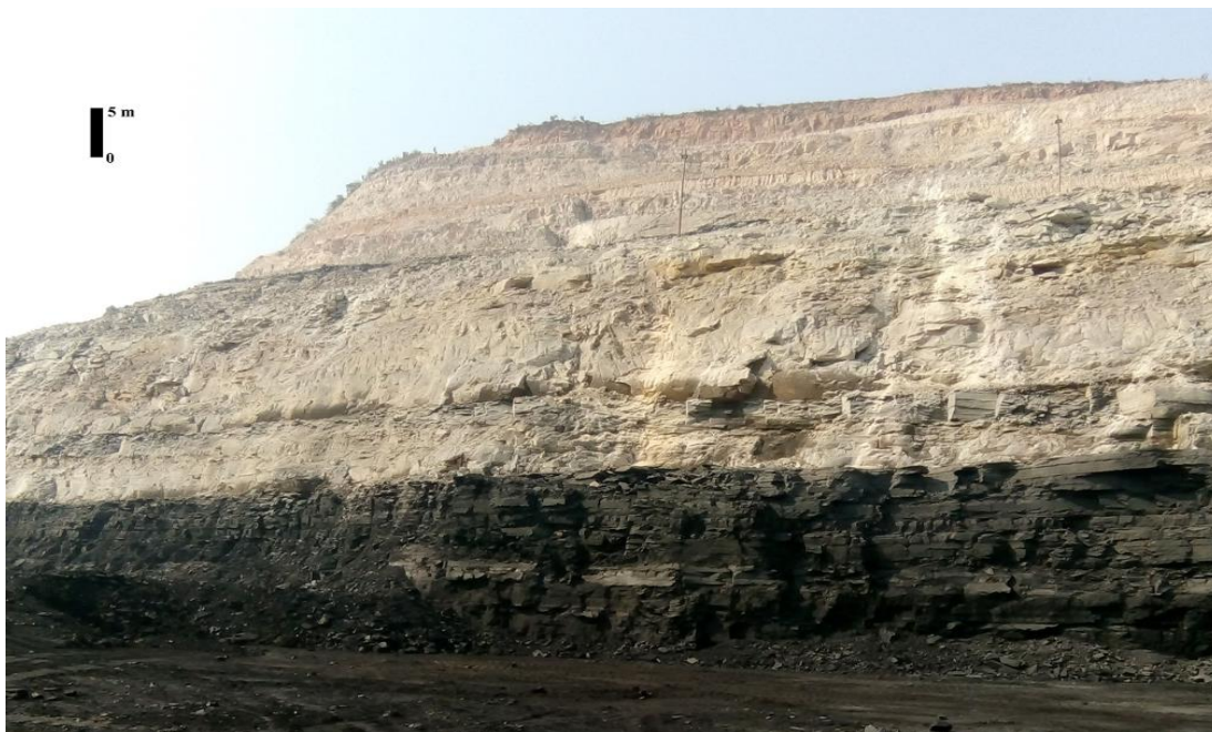
Figure 3.5. Vertical profile of working face of Dudhichua Mine showing exposure of Turra seam.
