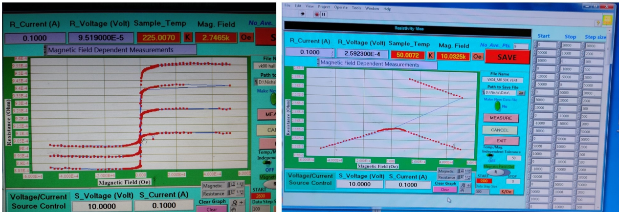
(a) Front panel for Hall measurement (b) Front panel for magnetoresistance measurement
