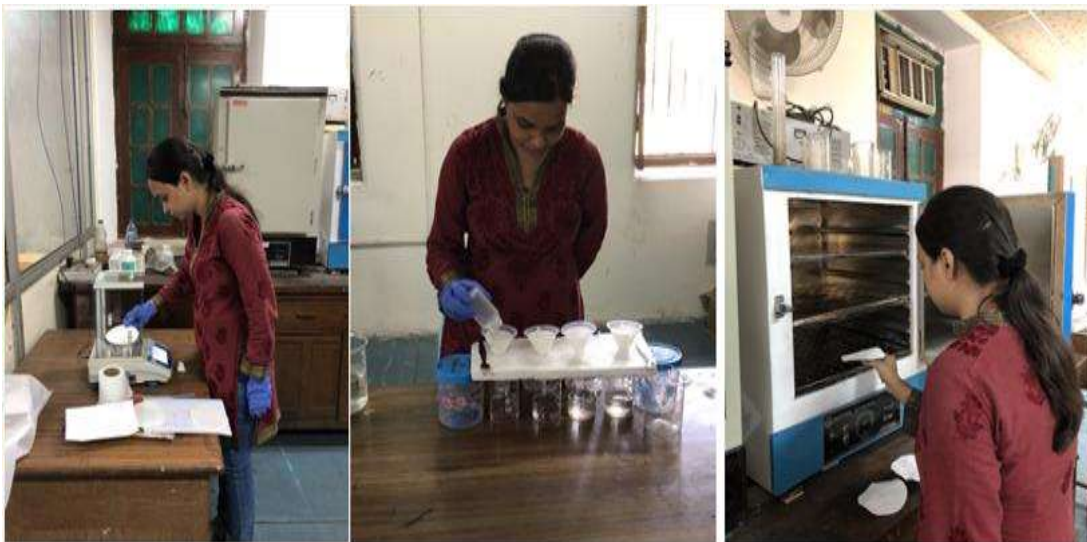
Fig 4.5 Laboratory analysis of water samples for Total Suspended Solids
