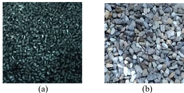
Fig. 3.3 Materials used in the study: (a) plastic granules, (b) stone aggregates.
