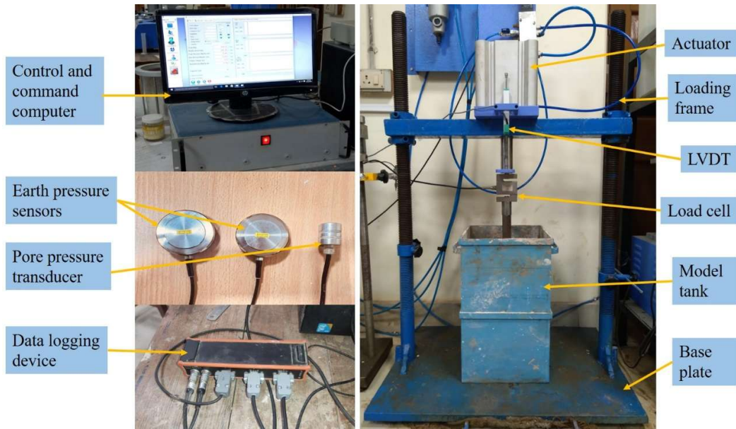
Fig. 3.10 Model test setup along with data loggers, earth pressure cells, and pore pressure transducer.
