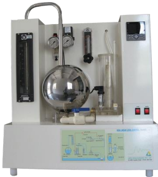
Figure 5. 1 Experimental setup of Conical Tank Process
