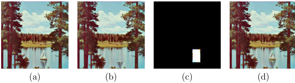
FIGURE 4.12: (a)Watermarked image of Boat_RGB image (b) Object removal attacks (c) tampered detected area (d) Recovered image.
