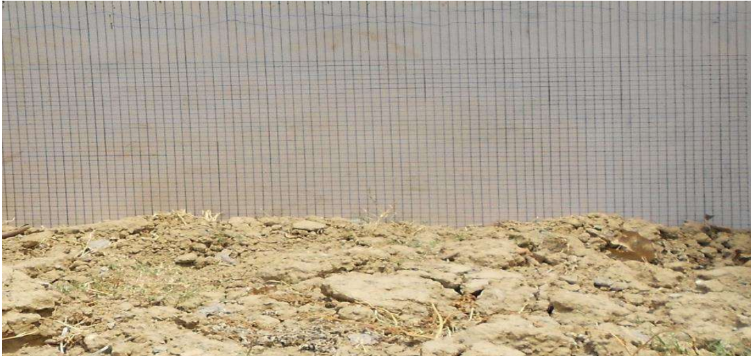
Figure 2.3 Metallic plate (1 meter long) used for the measurement of soil surface roughness
