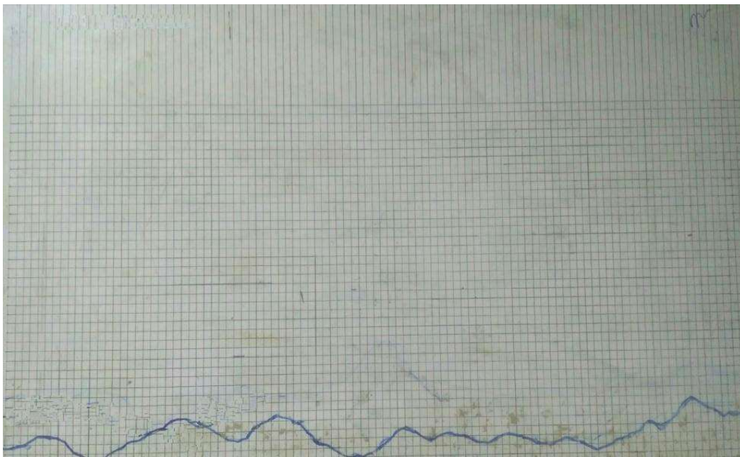
Figure 2.4 The surface roughness profile drawn on the metallic plate using ink marker
