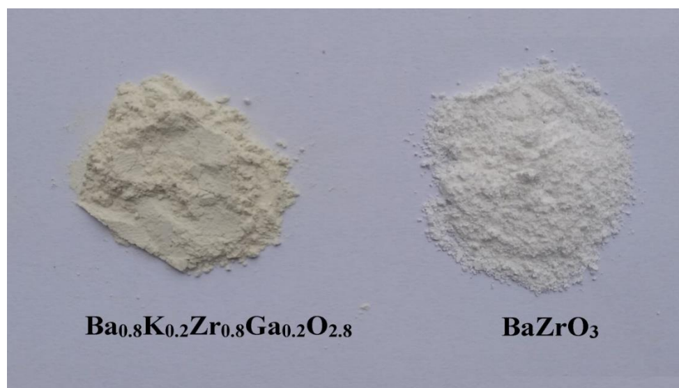
Figure 4.1 Photograph of synthesized powder (off-white colour) & \text{BaZrO}_3
