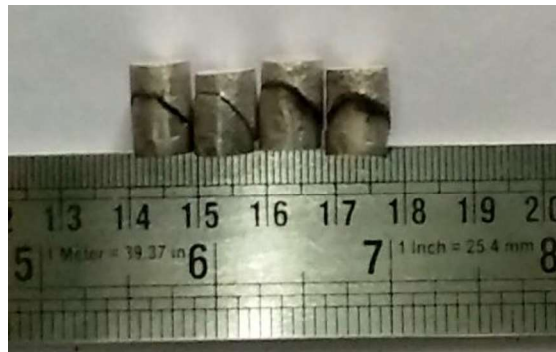
Figure 5. 13: Fractured samples in a compression test
