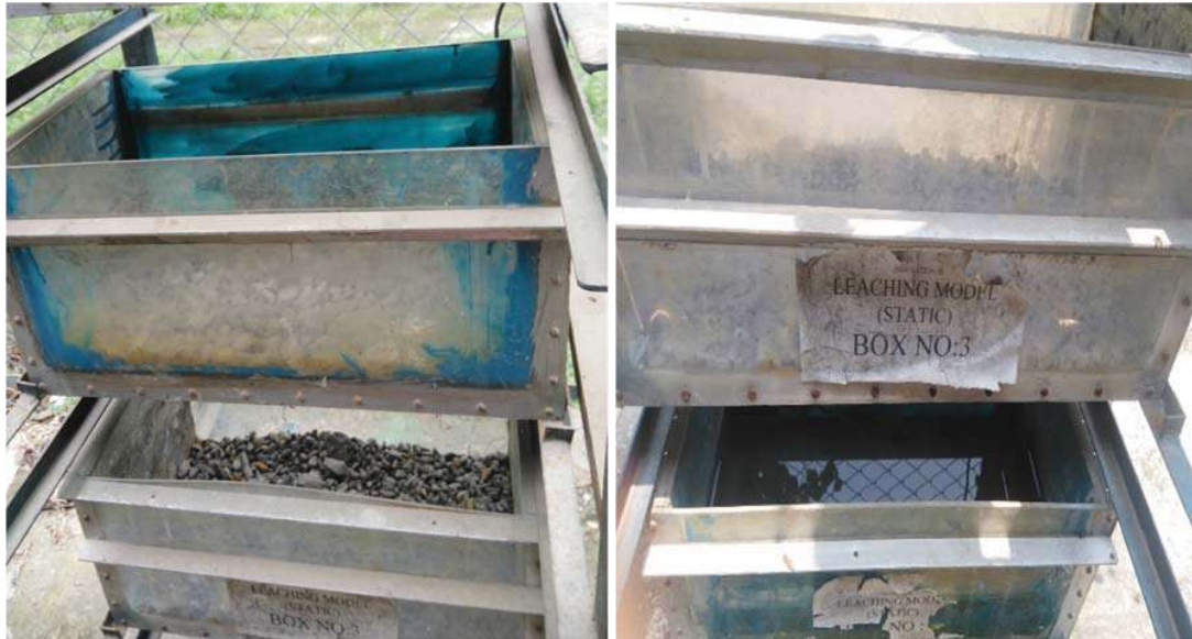
Fig. 4.26: Rain water passing through different litho- types of overburden
