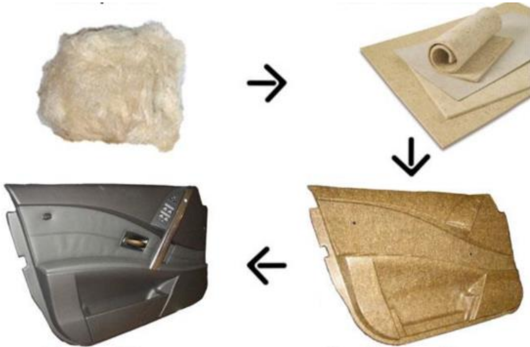
Figure 1.8. Manufacturing of door from hemp fibre [24].
