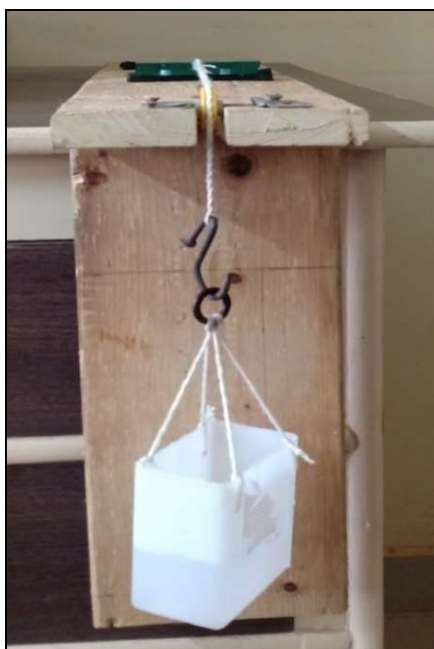
Figure 2.1 Apparatus for measurement of the spreadability of nanoformulation
