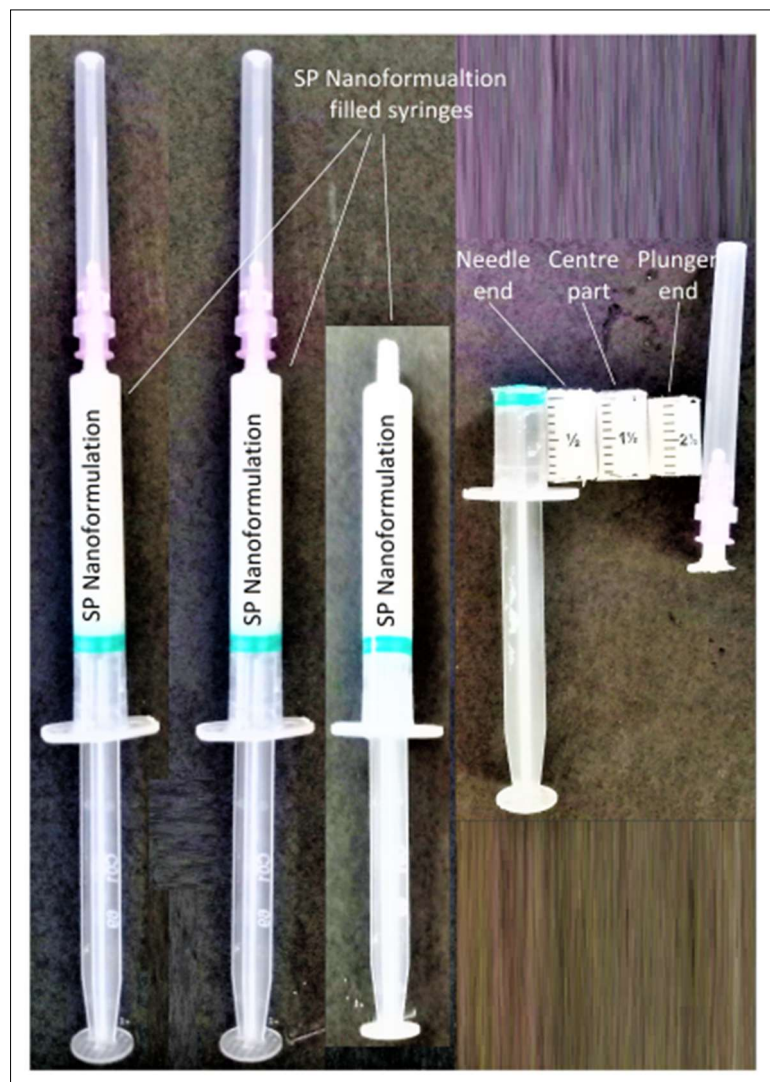
Figure 2.2: Content uniformity test. SP nanoformulation filled syringe tubes, tube was cut into pieces and content was evaluated for uniformity.
