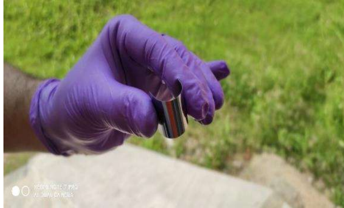
Fig.1.18: The developed \sim 30 \mu\text{m} thin flexible c-Si wafer by alkali etching during the research work.
